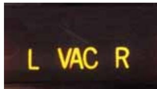
*Simple annunciator lights like this make it much easier to recognize a vacuum pump failure. If you fly regularly at night, or in IMC, consider them essential.*
