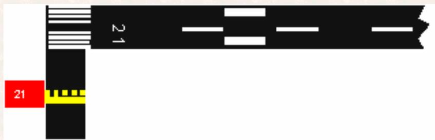
Runways with non-precision instrument approaches are similar to the VFR runway with the addition of threshold markings.
