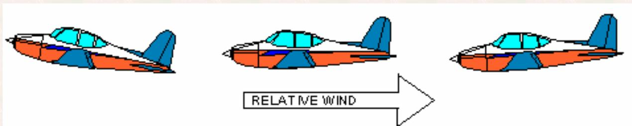
*airspeeds*. Maintaining a fixed altitude at a given airspeed requires the pilot to control two factors; (1) *Angle of Attack* and (2) *Power*. The angle of attack is controlled by the up, neutral, or downward trim position of the elevators. The power, is controlled by the "power setting" of the engine and propeller. For a "fixed pitch" propeller, this means adjusting the engine RPM. For a variable pitch propeller, this means adjusting both the throttle and the propeller pitch control.
