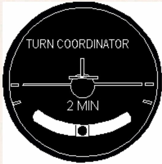
There are 2 marks on each side. The upper ones indicate level flight when the wing align with them. The lower marks indicates a bank angle of 15 degrees, which produces a standard rate turn. When the aircraft turns right, the miniature aircraft in the instrument indicated a right bank. When turning left, it indicates a left bank.
