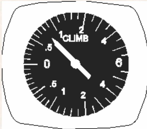
In small piston engine powered aircraft, the rate of climb will usually be less that 1000 feet per minute. Usual rate of decent enroute or approach to landing will be in the 500 feet per minute range. When flying straight and level, the instrument should indicate zero. Also when sitting stable on the ground the instrument should indicate zero. Most instruments are equipped with a small adjusting screw to calibrate the zero position when the aircraft is at rest on the ground.
