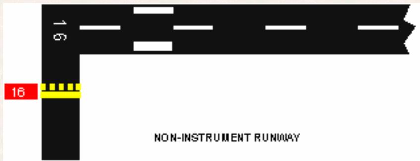
The runway threshold shown identifies a VFR only runway. It contains a runway number and an aiming point marker on each side.
