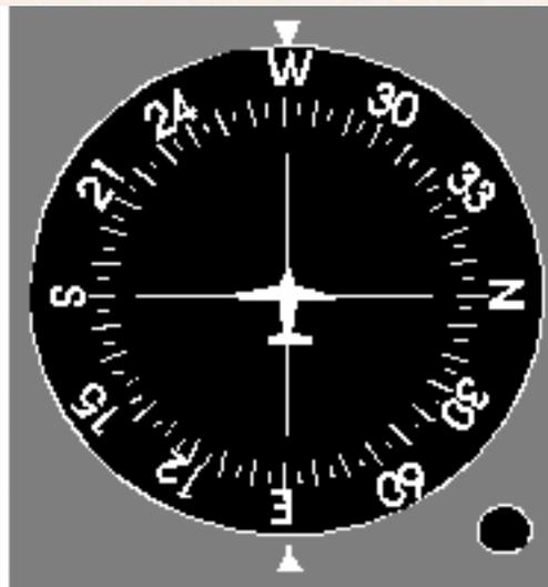
The HI is not automatically synchronized with the magnetic compass. It must be set to the compass heading while level on the airport surface prior to take-off.
